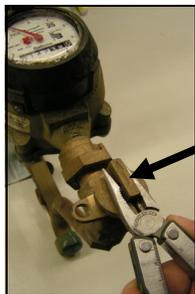
Arrow in line with meter, **ON**, arrow not in line with meter, **OFF**. Valve will turn easily.
