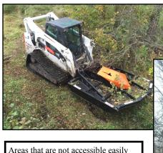
Areas that are not accessible easily can be cut and shredded rather easily with a properly equipped skid loader. Being able to access lines is important to proper maintenance and repair for all utilities.
